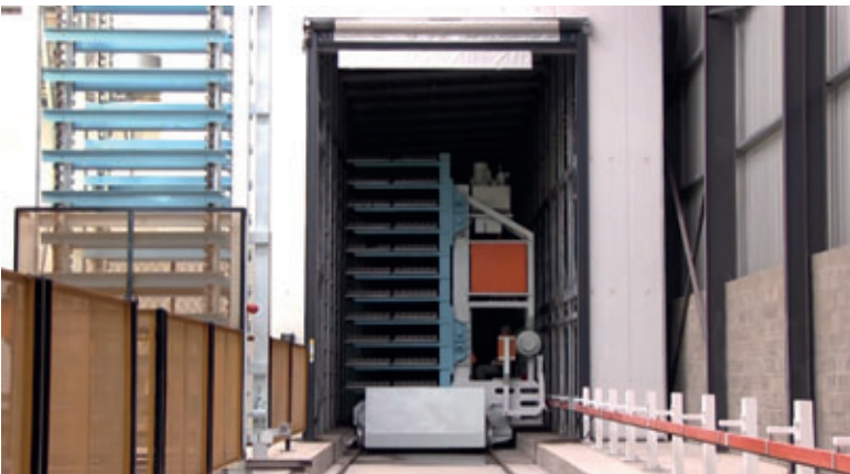
Fast operating tarp door – an economical and simple solution for quick opening and closing allowing uninterrupted transfer car operation with minimal heat and moisture loss from the single atmosphere curing chamber.
