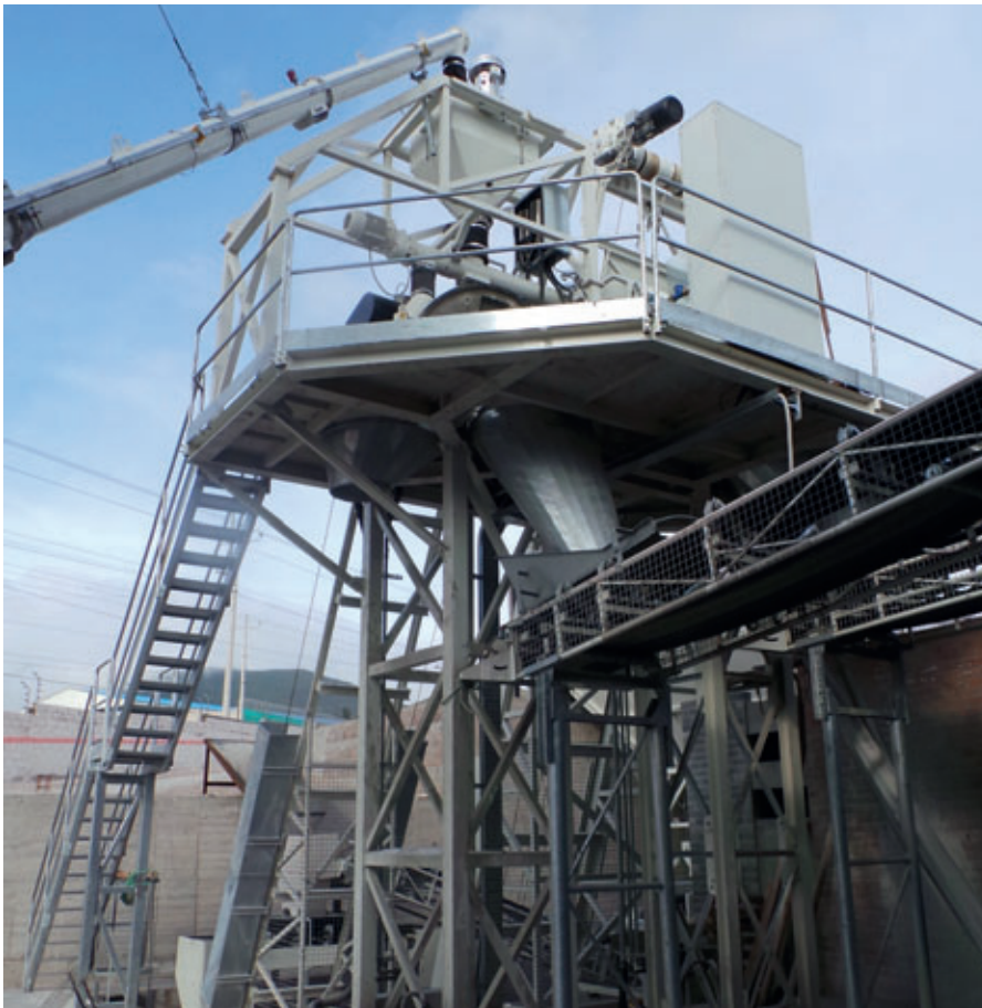
Euromecc mixers platform and belt conveyor for feeding the Multilayer machine
