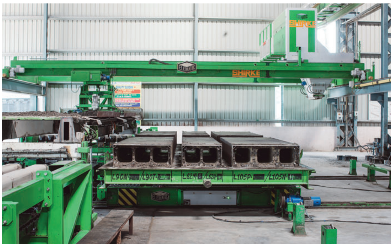
The '3S' column is a unique product of Shirke, having hollow cores and relatively new technology for Elematic. The molds for B.G Shirke were developed based on a previous machine model for a similar hollow core product.
