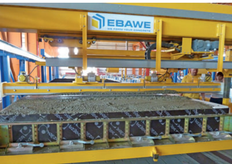
The freshly poured concrete is drawn off to the desired level and compacted with a vibrating levelling beam.
