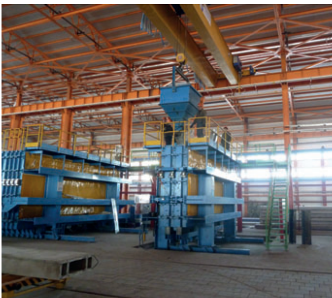
Battery mould for production of partition walls
