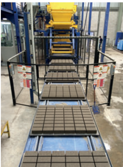
Fresh paving stones are leaving the block making machine XL 9.1
