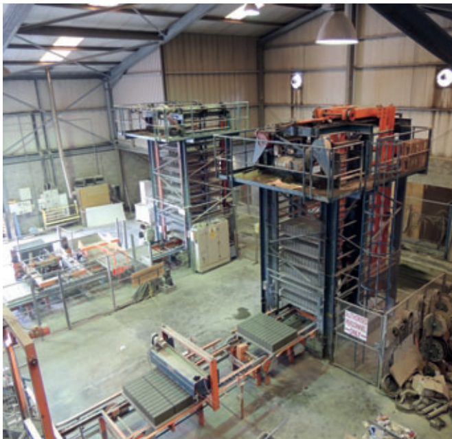
Before: elevator & lowerator area with raised maintenance platforms
