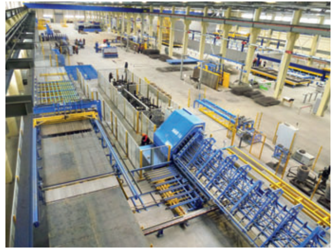
The required reinforcement meshes are produced just in time by the fully automatic M-System Evolution mesh welding machine. The machine receives the required CAD data from ebos.
