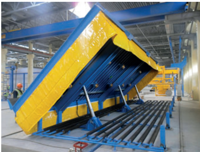
The new plant in Uljanovsk also has two tilting tables, which are equipped with a compaction and heating system.
