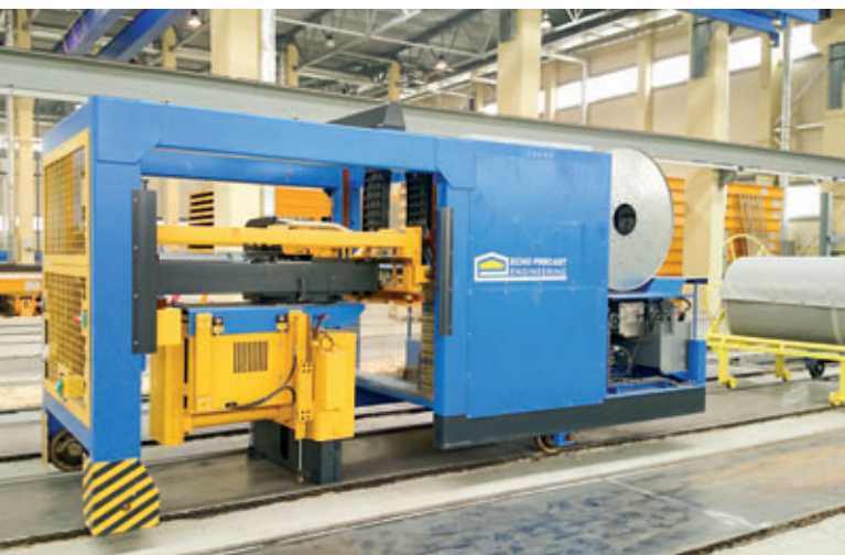
The cured concrete elements can be shortened to the desired length with the aid of the multi-angle sawing machine.
