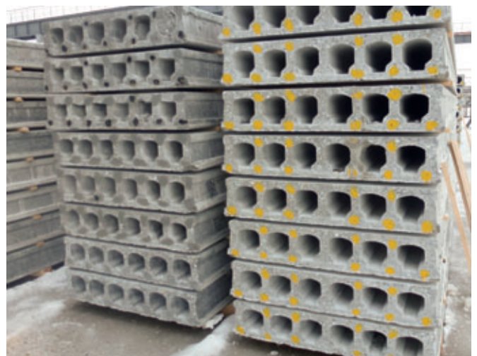
The finished prestressed hollow-core slabs are stored outside, waiting to be loaded and taken to the building site.
