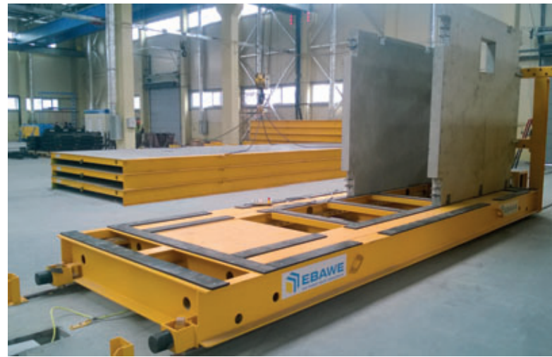
The precast concrete elements are transported into the outdoor store by a run-off truck.
