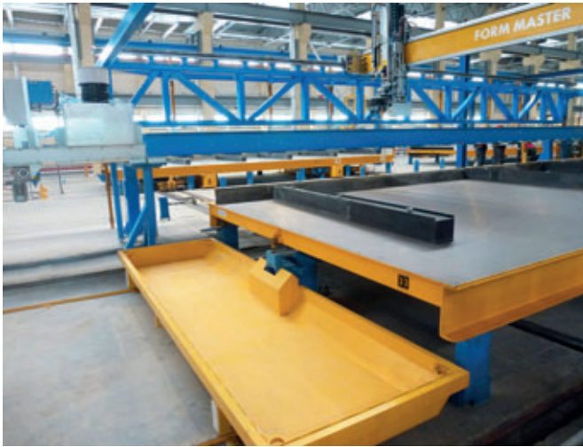
With the Form Master robot system the shutters are fully automatically removed after the completion of a production cycle, supplied to a shutter cleaning unit and placed precisely on the pallet shuttering surface again for the new occupation.
