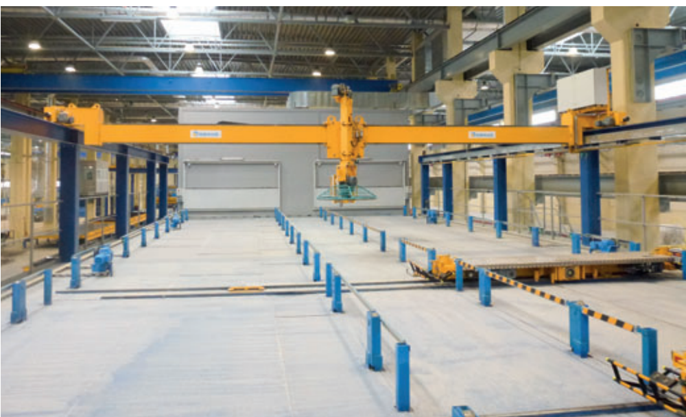
Following the pre-curing of the concrete in the pre-curing chamber the pallets are moved by the lifting transfer table to the 2nd level. A power trowel and four smoothing stations are available there for the fine smoothing.
