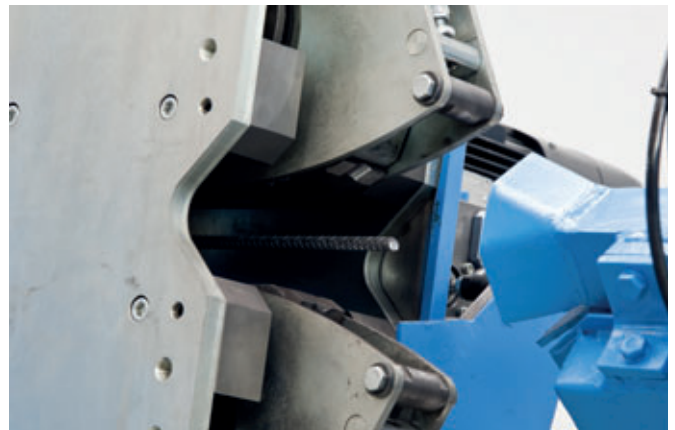
Fig. 4: The flying shear guarantees accurate and fast processing.
