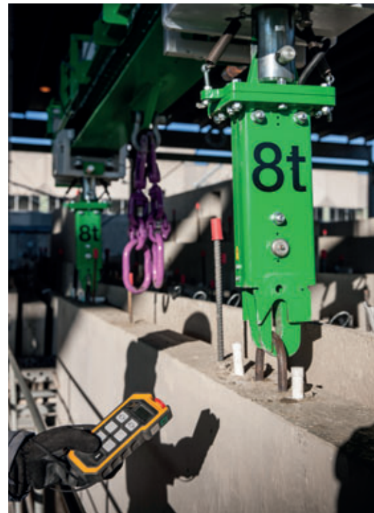
Time-consuming chain mounting is not needed as the Elematic lifting beam is equipped with lifting hooks
