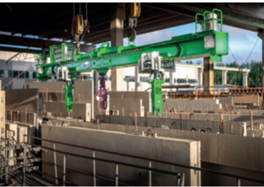
Elematic E9-16-5a lifting beam has been developed to help improving work site safety
