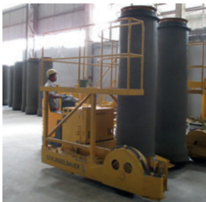
The second member of personnel responsible for pipe production moves the freshly-made products to the curing area, using a removal truck.
