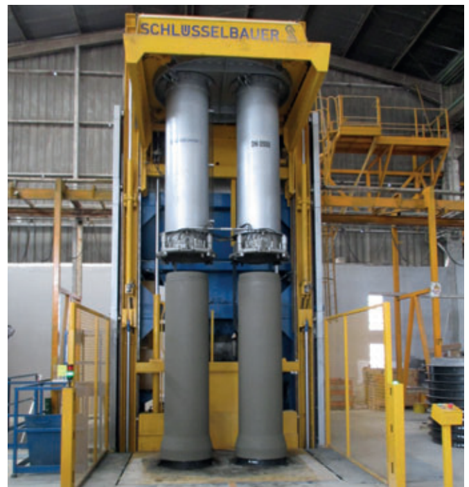
The Precise system, supplied by Schlüsselbauer Technology, can be used for single and twin production. Two concrete pipes are manufactured at SCG in a – even by international standards – remarkably short cycle time.
