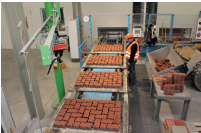
Directly after the separation the two transport lines of the two lowerators join together to form a single line.
