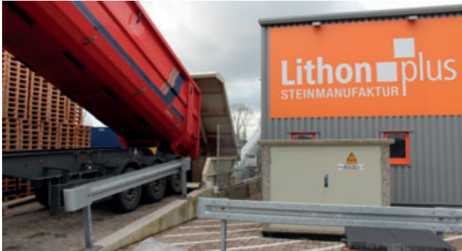
On delivery the aggregates are tipped directly from the truck into a 22 m 3 feed silo.
