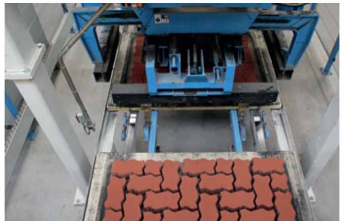
In this station the stones are pushed together on the underlay board.
