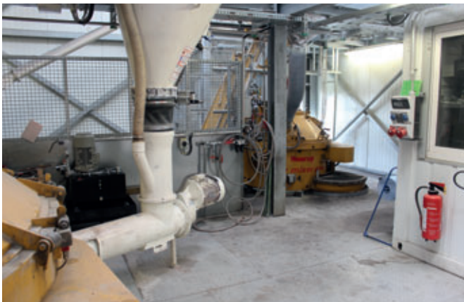
In ubo Engineering's concept, water and cement are guided downwards into the mixer.
