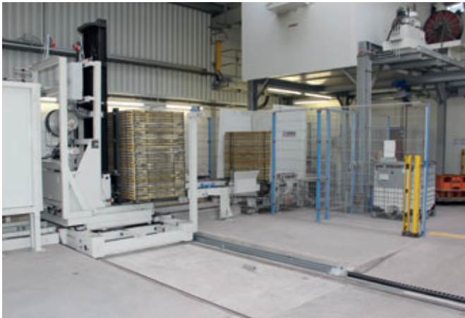
The finger car of the board buffer rack also supplies the concrete block making machine with the Assyx underlay boards.
