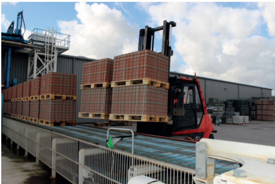
The fork-lift truck that takes the stone packages to the outdoor storage area is equipped with a double fork with which it can take two double packages at once, i.e. a total of four stone packages.
