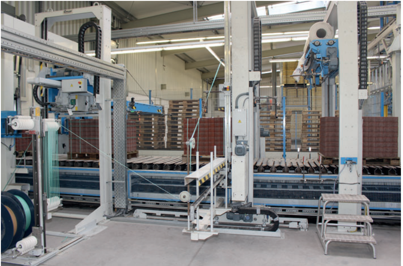
The finished stone packages are finally strapped horizontally and vertically and then transported into the outdoor area of the hall.
