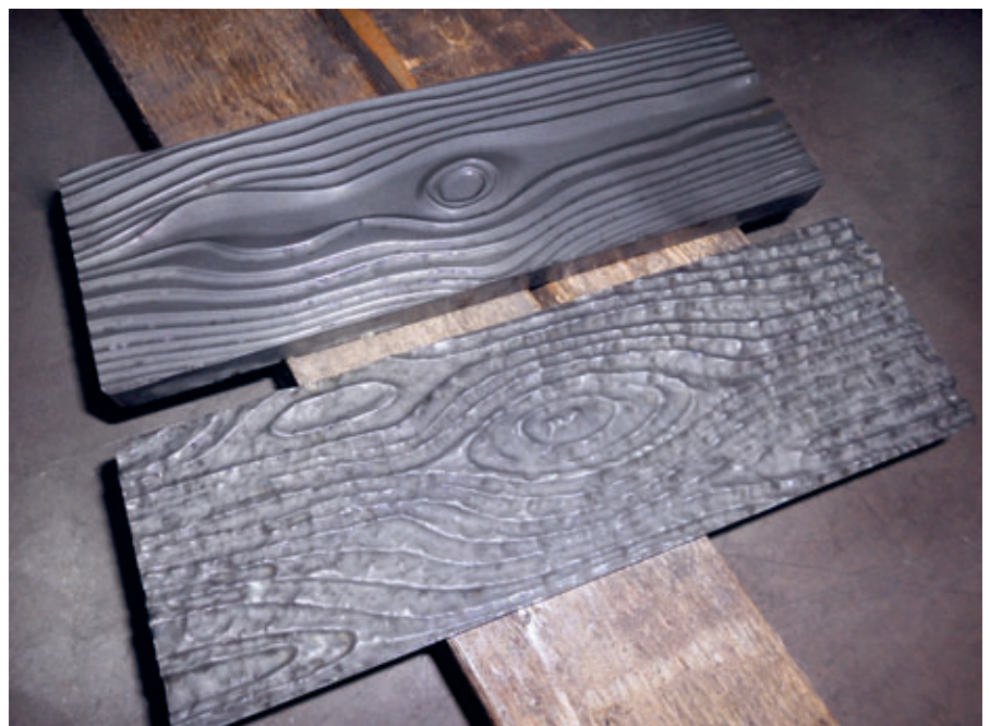
Sample tamper shoe for real test production in an existing concrete block mould.
