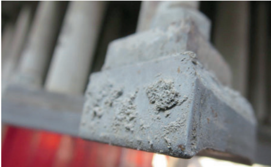
Typical wear patterns: one-sided chamfer wear
