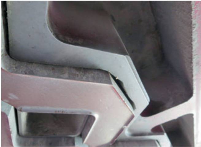
Elephant's feet" at the lower edge of the mould bottom
