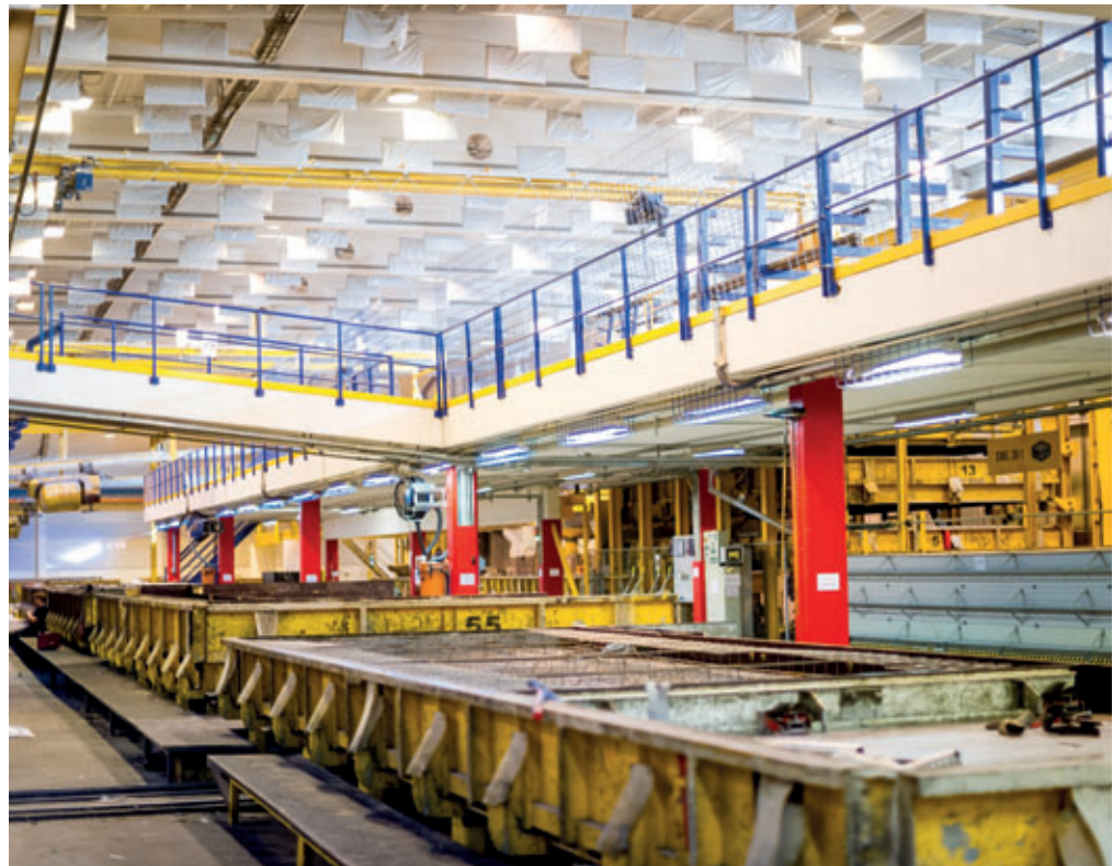
Production output for the entire factory is typically 750 tonnes/day, drawing upon the solid capabilities of EliPlan since 2002. For façade production alone, the factory has 25 tables (10 m x 4 m), each able to cast up to 450 mm thickness.
