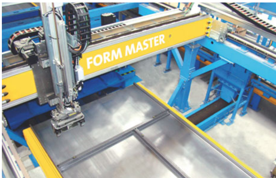
The new Infinity Line shuttering system, developed and patented by the Progress Group, enables the gap-free shuttering of precast concrete elements practically without the use of polystyrene extensions.
