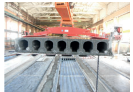
Takeoff of the finished hollowcore slabs
