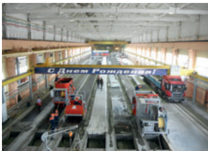
Echo Precast Engineering has delivered equipment for the production of prestressed hollowcore slabs for the production site of SU-155 in Domodedovo.
