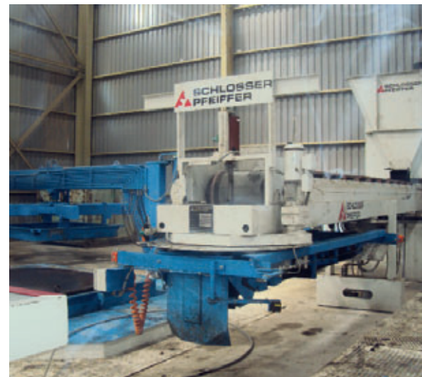
Variant 4000: universal machine for large pipes and box culverts at Sarl Etber, Bouira
