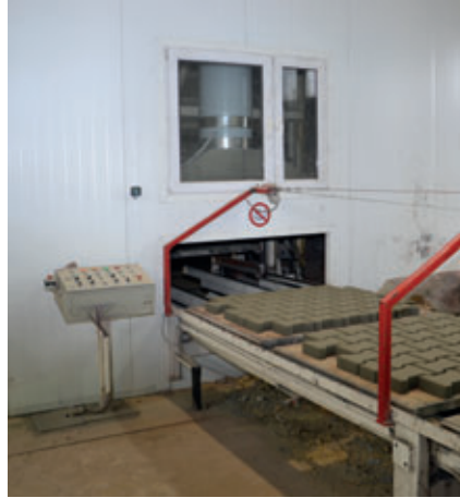
Curing Chamber Wet-Side-Entry / Dry-Side-Exit for fresh/hardened concrete products; including window, insulated wall and exhaust with heated hood to prevent moisture from escaping into the production area and drips on fresh product
