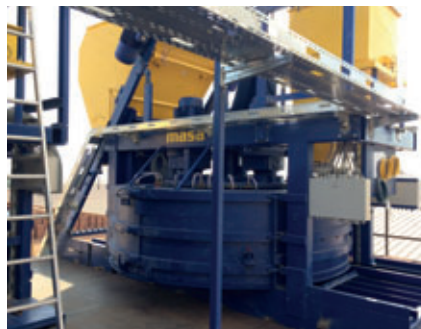
Final assembly of the Masa PH 3000/4500 mixer
