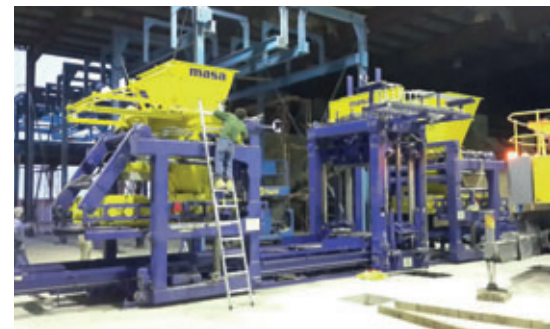
Assembly of the Masa XL 9.2 concrete block making machine
