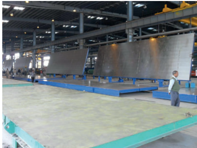
tecnocom supplied a total of 36 TTE tilting tables to the Amrapali Precast plant in the southeast of New Delhi.
