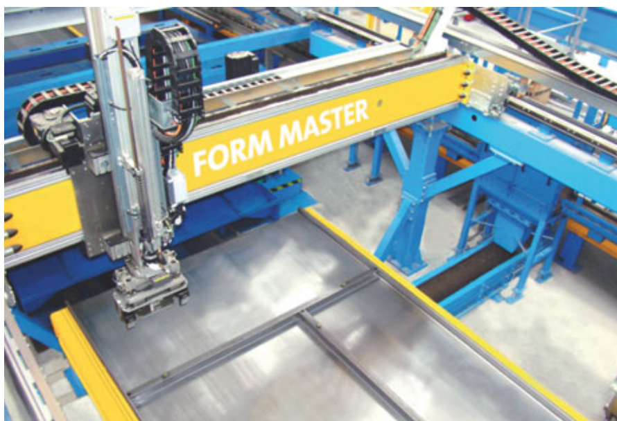
The new Infinity Line shuttering system, developed and patented by the Progress Group, enables the gap-free shuttering of precast concrete elements practically without the use of polystyrene extensions.
