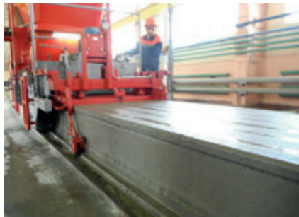
The slipformer can produce hollowcore slabs with a thickness of 6 to 60cm as well as piles, spandrel beams, road slabs etc.
