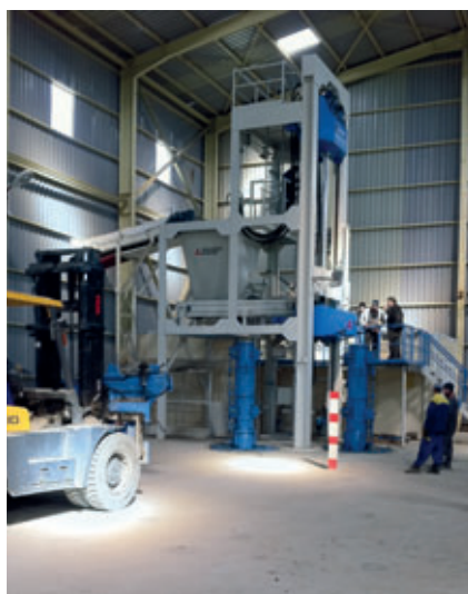
RP 1225 radial press: heavy-duty machine for drainpipes with integrated seal from DN 300 to 1200 mm, overall length 2.5 m, at Sarl Etber, Bouira
