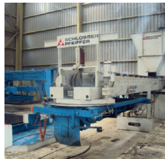
Variant 4000: universal machine for large pipes and box culverts at Sarl Etber, Bouira
