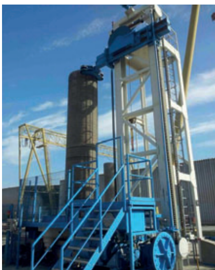
Vertical prestressing machine in the Hydroamègement Rouiba plant in Algiers for the winding of core pipes from DN 600 to DN 2000, overall length 6 m.
