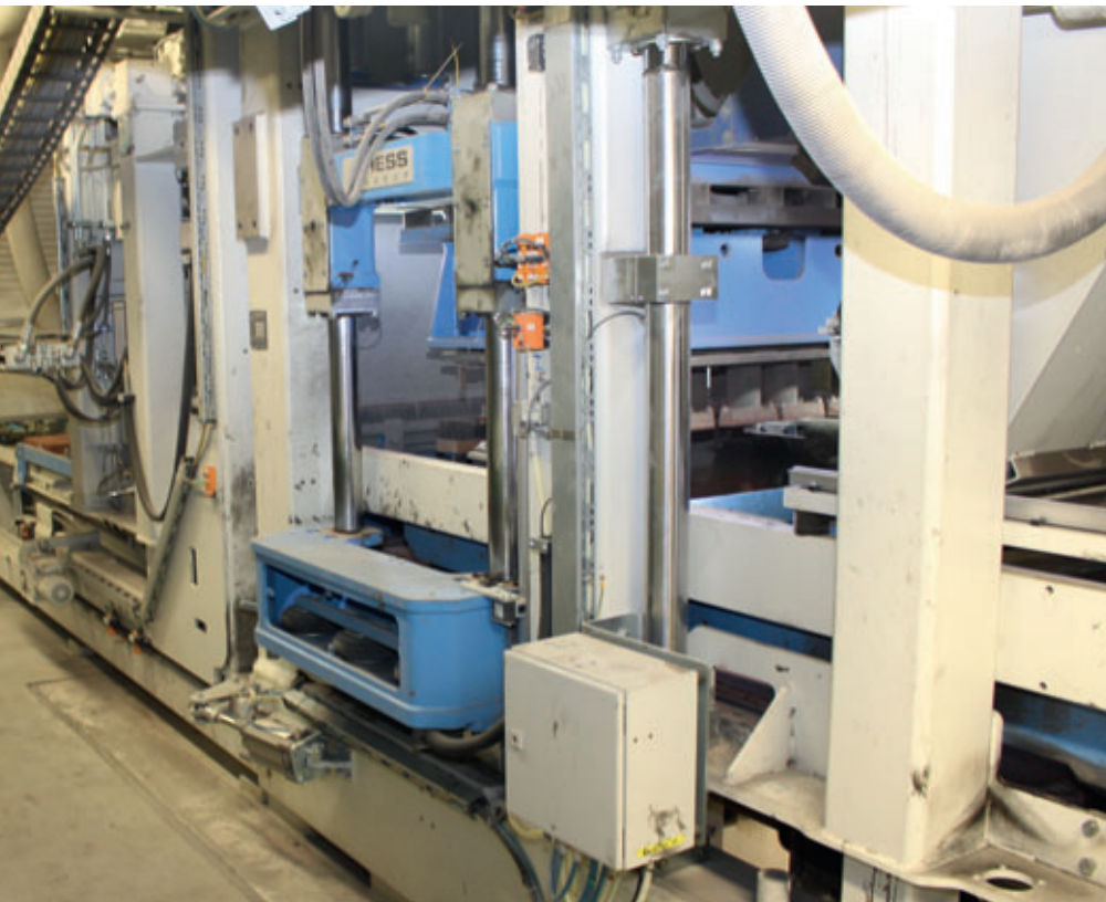
3 rd Hess RH 2000-3 MVA, production pallet size 1450 x 750 mm, commissioned at the start of 2014
