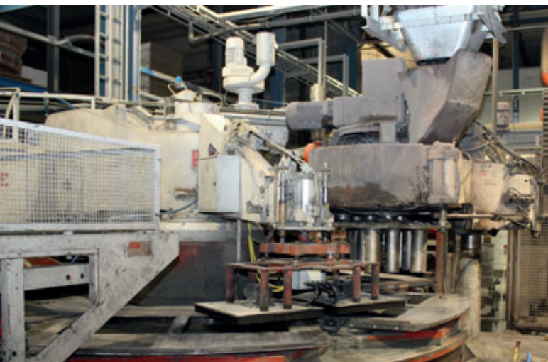
Hermetic turntable press with a pressing force of 14,000 kN from SR-Schindler
