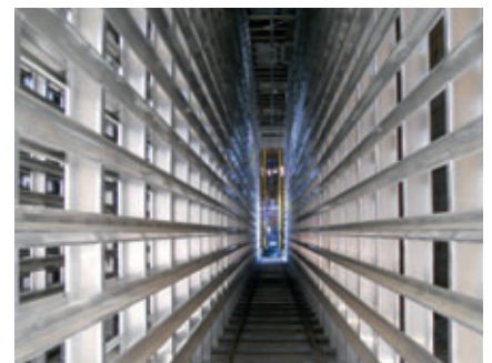
In total, the rack system measures 26,300 x 21,280 mm and has an overall height of 9,500 mm.
