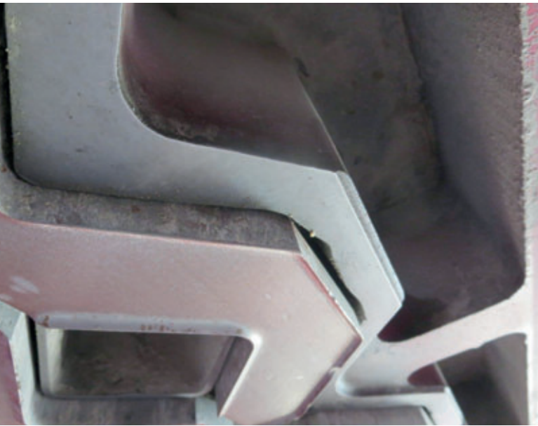
Elephant's feet" at the lower edge of the mould bottom
