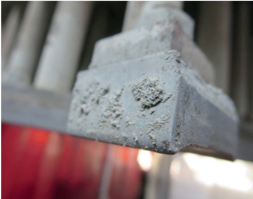
Typical wear patterns: one-sided chamfer wear
