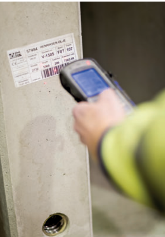
Keeping track of finished products is easy and simple, thanks to the barcode system that EliPlan enables.
