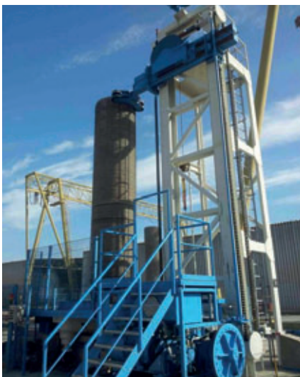
Vertical prestressing machine in the Hydroaménagement Rouiba plant in Algiers for the winding of core pipes from DN 600 to DN 2000, overall length 6 m.
