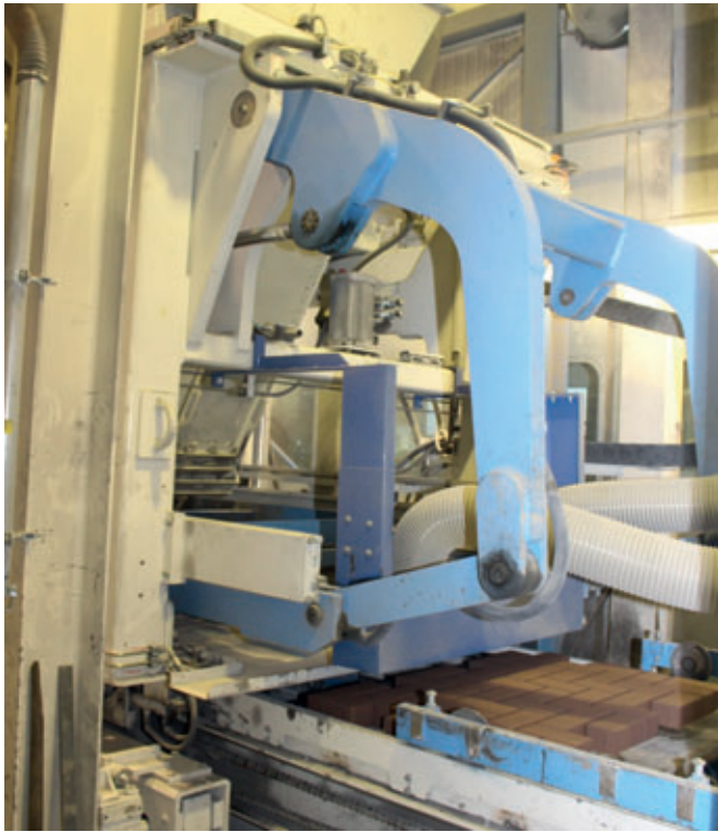
1 st Hess RH 2000-3 MVA, production pallet size 1450 x 1250 mm, commissioned in mid-2011
