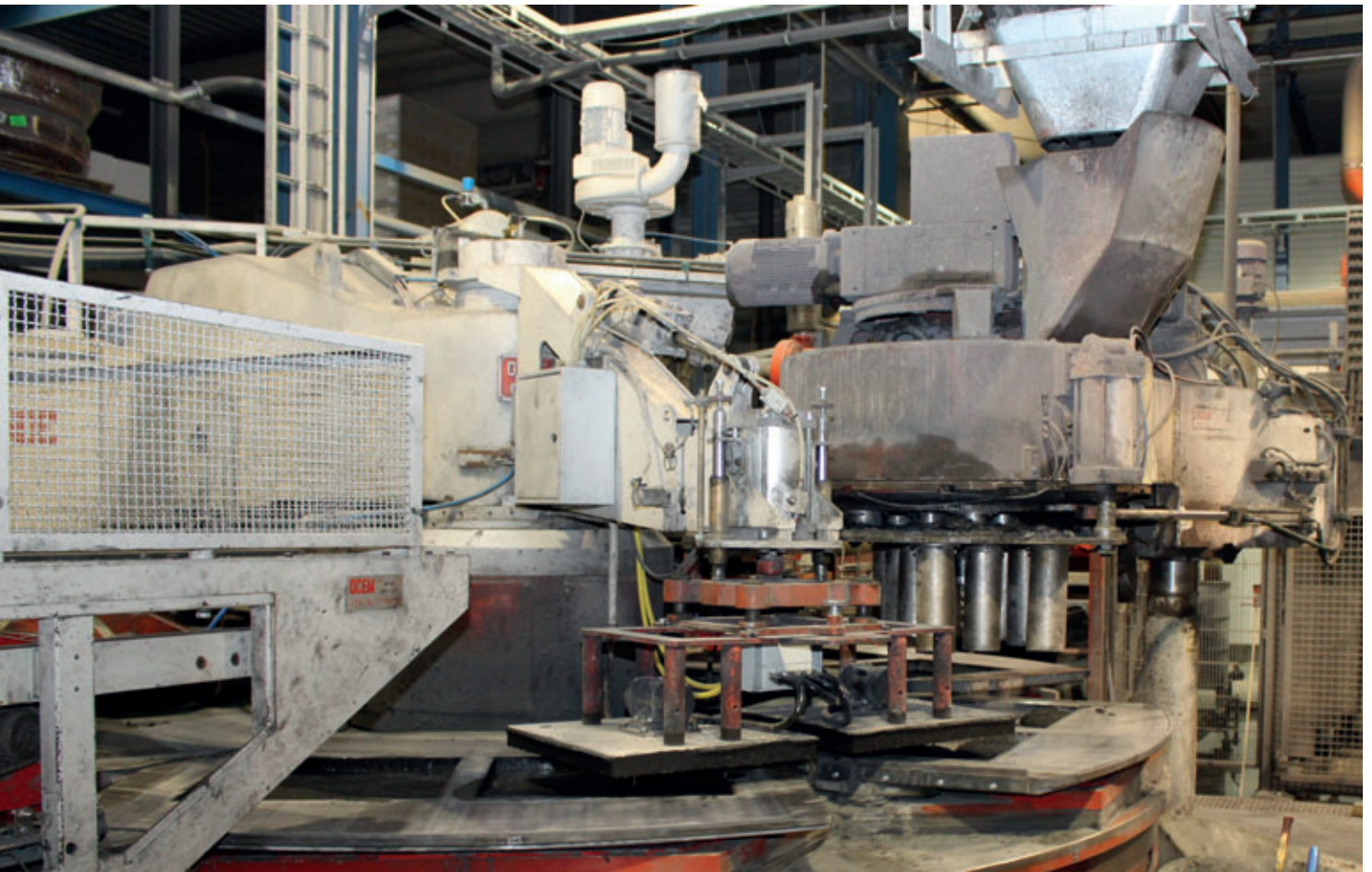
Hermetic turntable press with a pressing force of 14,000 kN from SR-Schindler
