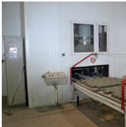
Curing Chamber Wet-Side-Entry / Dry-Side-Exit for fresh/hardened concrete products; including window, insulated wall and exhaust with heated hood to prevent moisture from escaping into the production area and drips on fresh product
