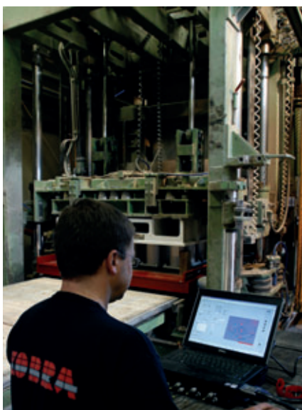
Recording and analysis of the processes during the compaction process with the aid of vibration measurements on up to 8 channels at the same time.
