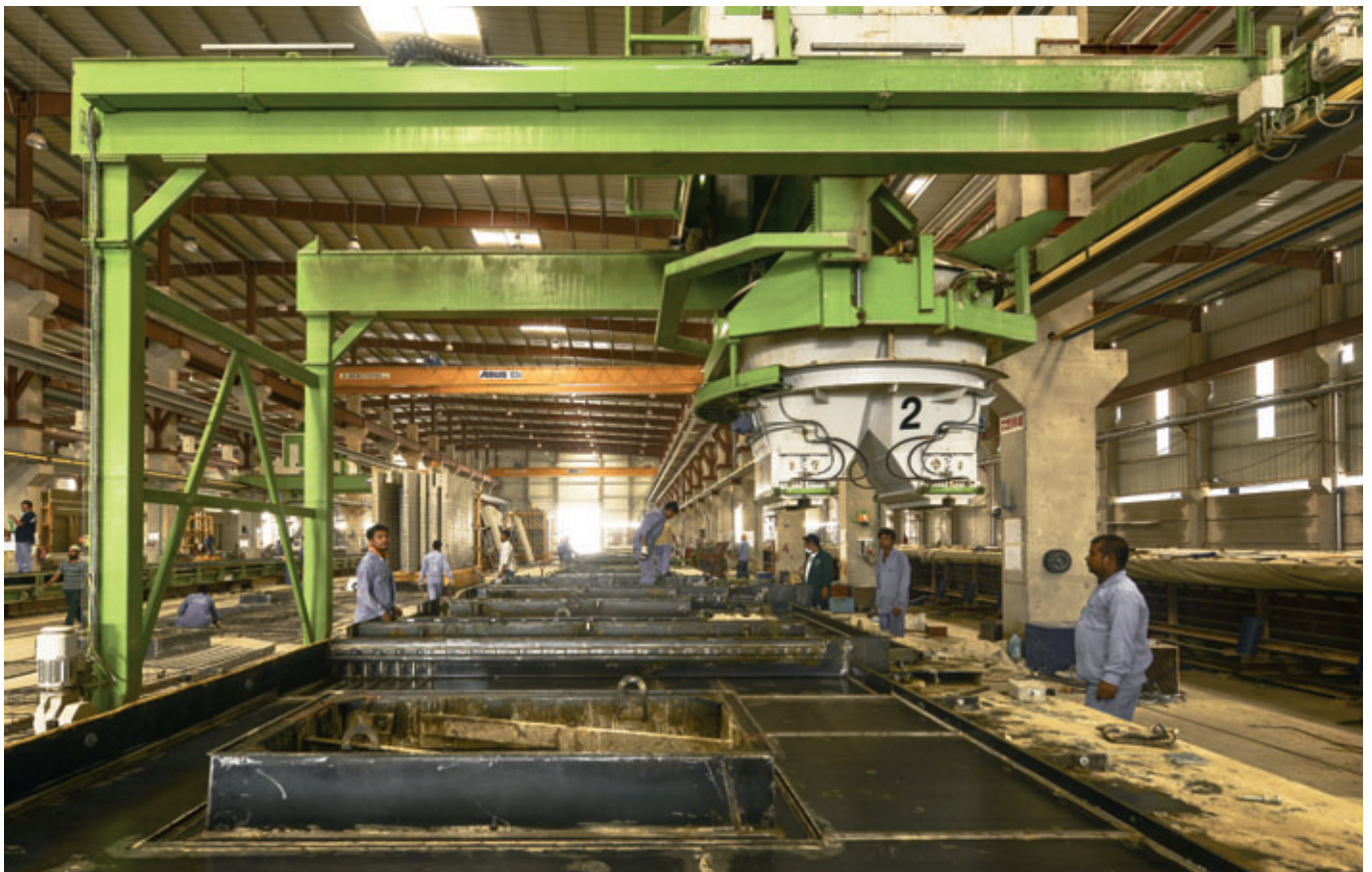
Casting machine at Alrashid Abetong
