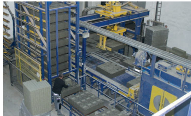
An employee inserts suitably pre-cut insulating material into the hollow chambers of the Jasto Plan Therm blocks.
