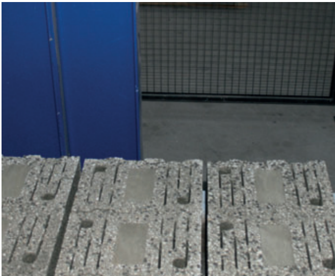
Before packaging, the block layers are slightly separated so that the subsequent stone packages can be better aired.
