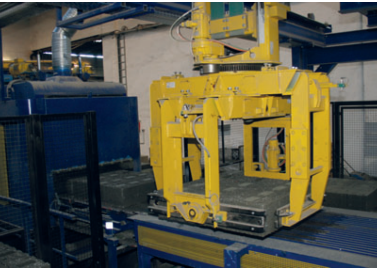
The gripper takes the blocks in layers from the steel sheets and sets them down in front of the grinding unit.
