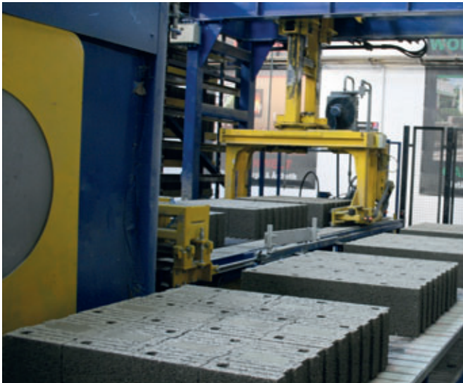
After milling, the blocks are placed on the slat conveyor, which takes them to the packaging area.
