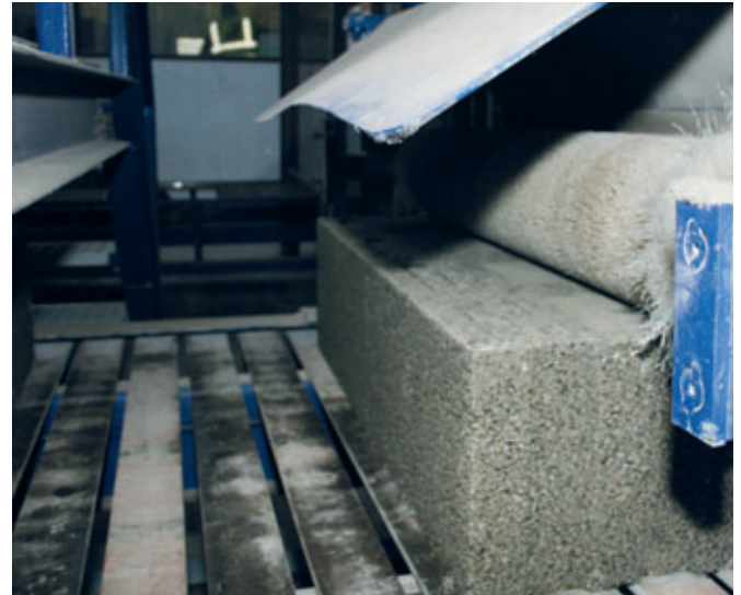
Final brushing of the surface for the removal of any milling residues
