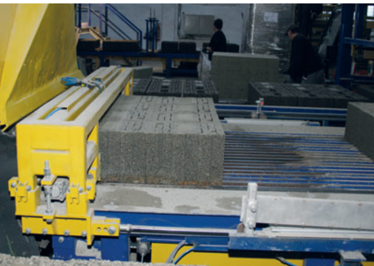
Jasto Plan Stones are milled to a height of 24.9 cm. Jasto Klassik Stones in contrast are manufactured with a height of 23.8 cm
