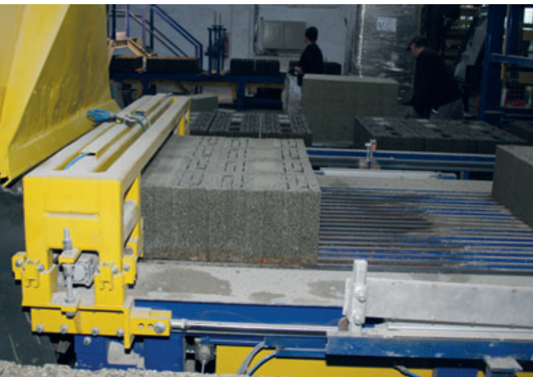
Jasto Plan Stones are milled to a height of 24.9 cm. Jasto Klassik Stones in contrast are manufactured with a height of 23.8 cm
