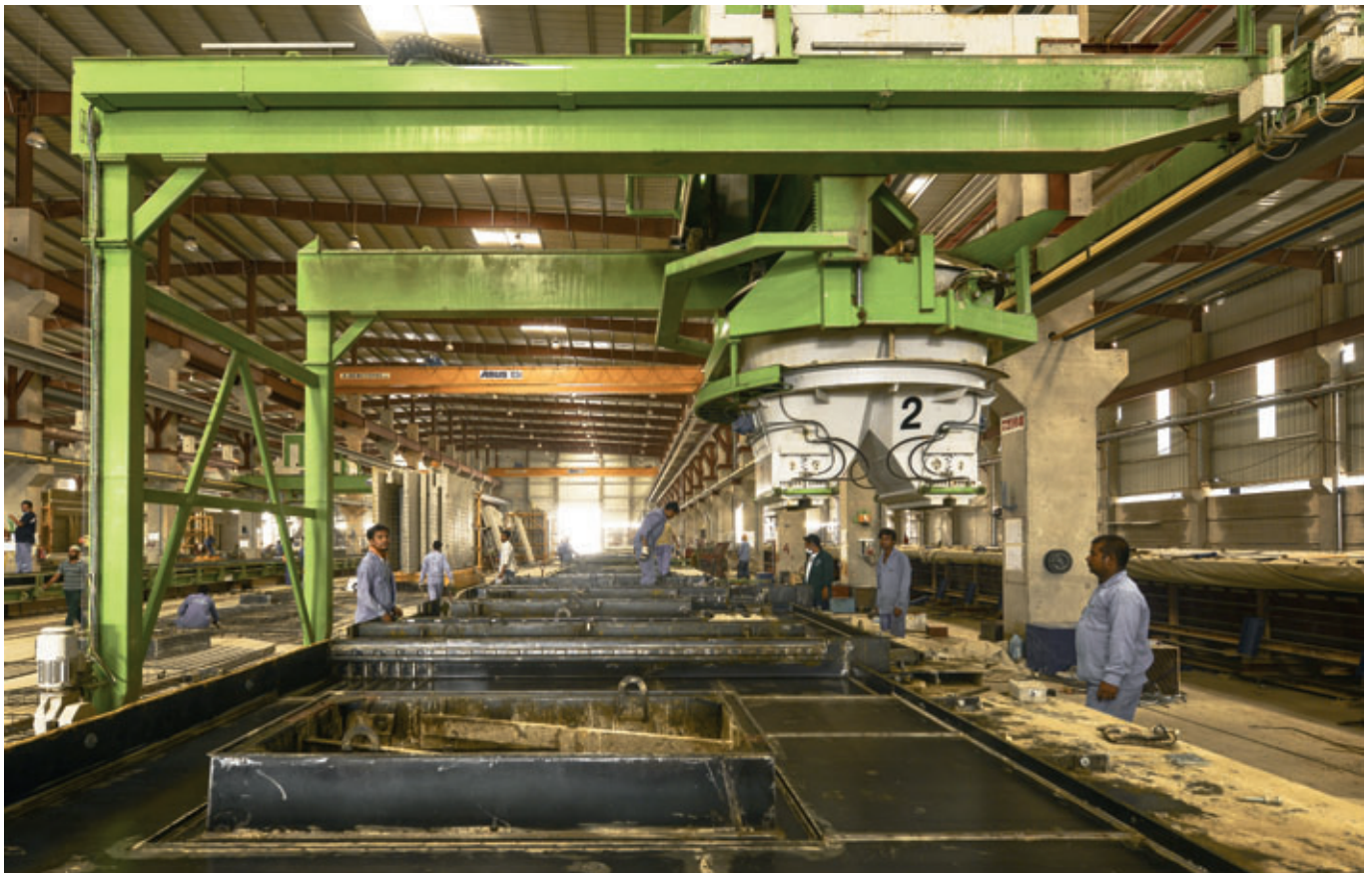
Casting machine at Alrashid Abetong
