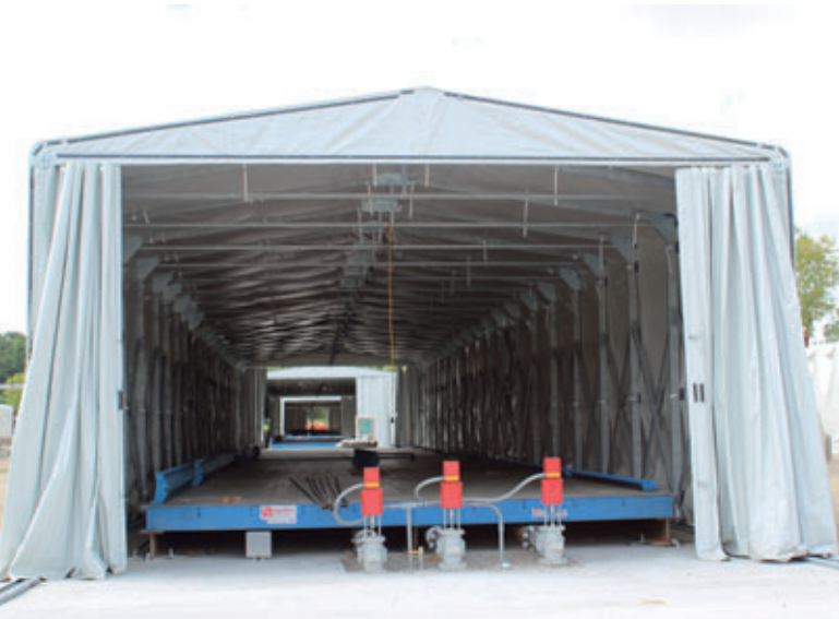
Heavy-duty valves distribute the vapor to the curing tables.
