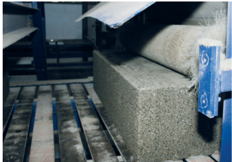
Final brushing of the surface for the removal of any milling residues
