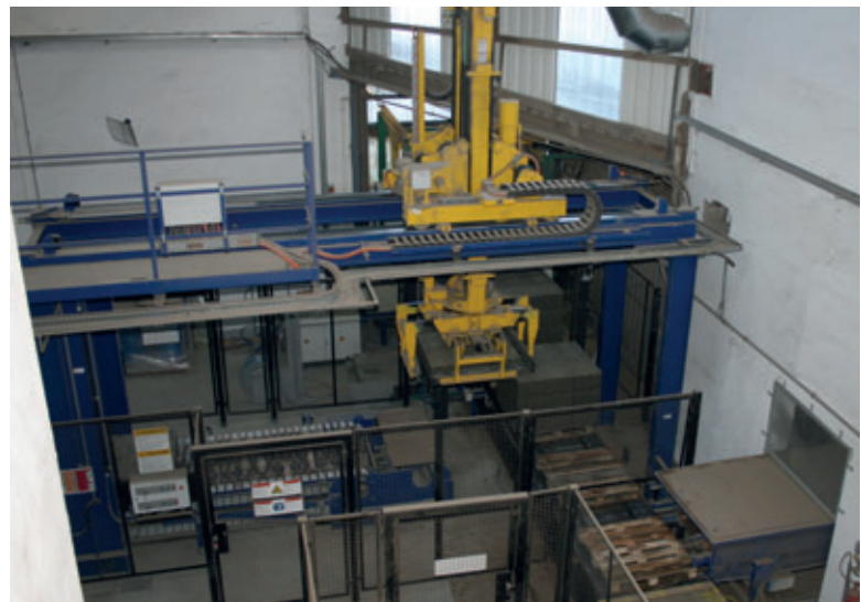
Packaging the pumice concrete blocks on wooden pallets
