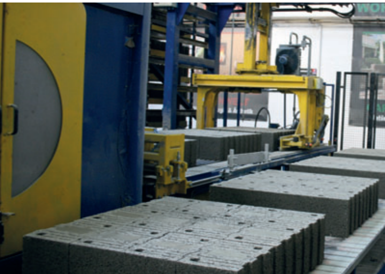
After milling, the blocks are placed on the slat conveyor, which takes them to the packaging area.
