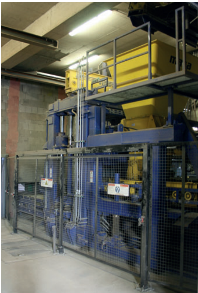
Masa XL 9.1 concrete block making machine
