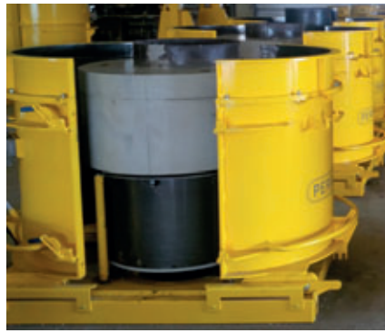
The height of the pre-cast components can be easily adapted in the wet cast moulds.
