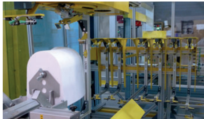
The negatives of the required channel components are accurately cut from EPS preforms using hot wire cutters.
