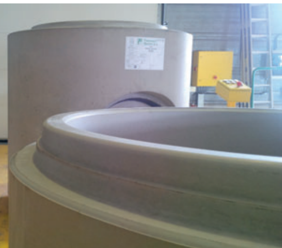
Immaculate concrete surfaces, including the spigot end.
