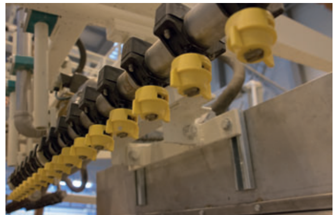
Nozzles of the Masa washing unit
