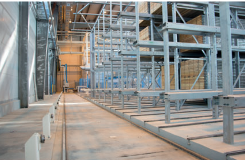
Depending on requirements the boards are either buffered or supplied to the production cycle
