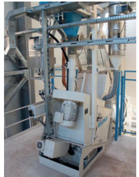
The concrete mixture for the facing concrete is manufactured by the Masa S 350/500 mixer
