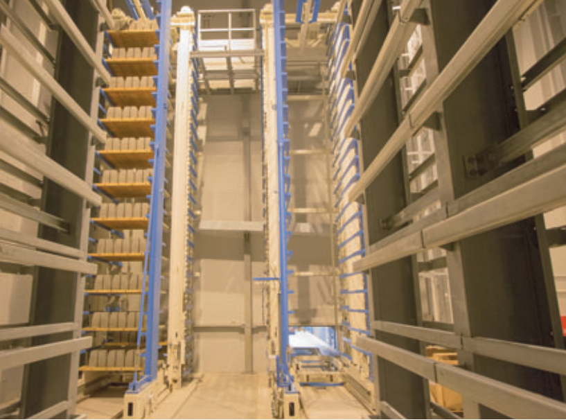
Two lowerators for two return transport routes
