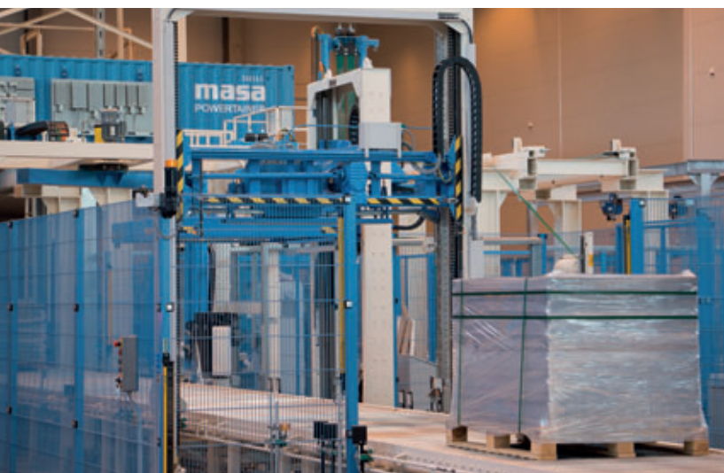
Well packed and ready for transport: foil wrapping plus vertical and horizontal strapping of the finished paving stones
