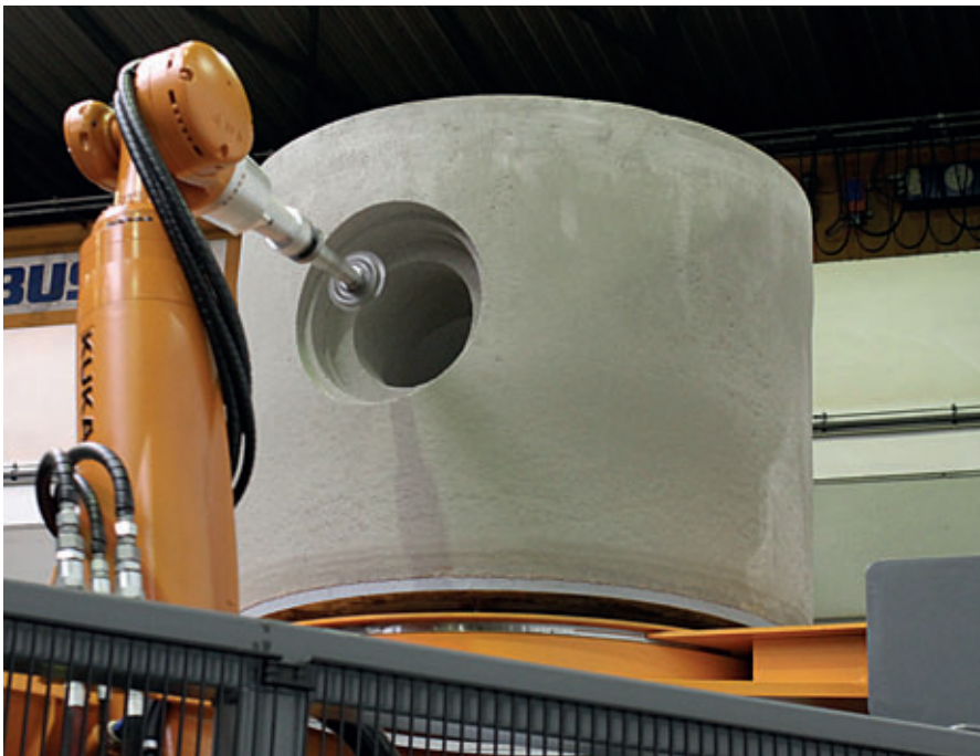
The Primuss concrete milling machine mills runs and channels in manhole bottoms with an accuracy of millimetres.
