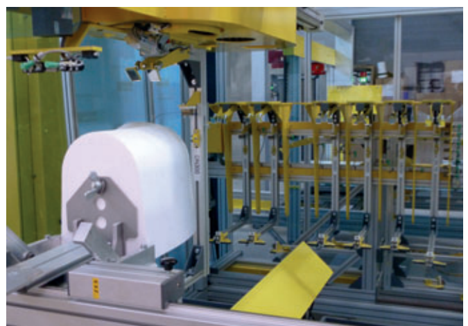
The negatives of the required channel components are accurately cut from EPS preforms using hot wire cutters.
