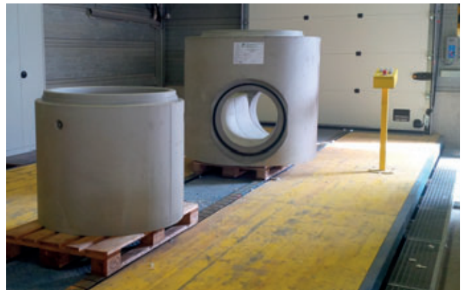
The first products with integrated seals – of impeccable quality – leave the manhole factory.
