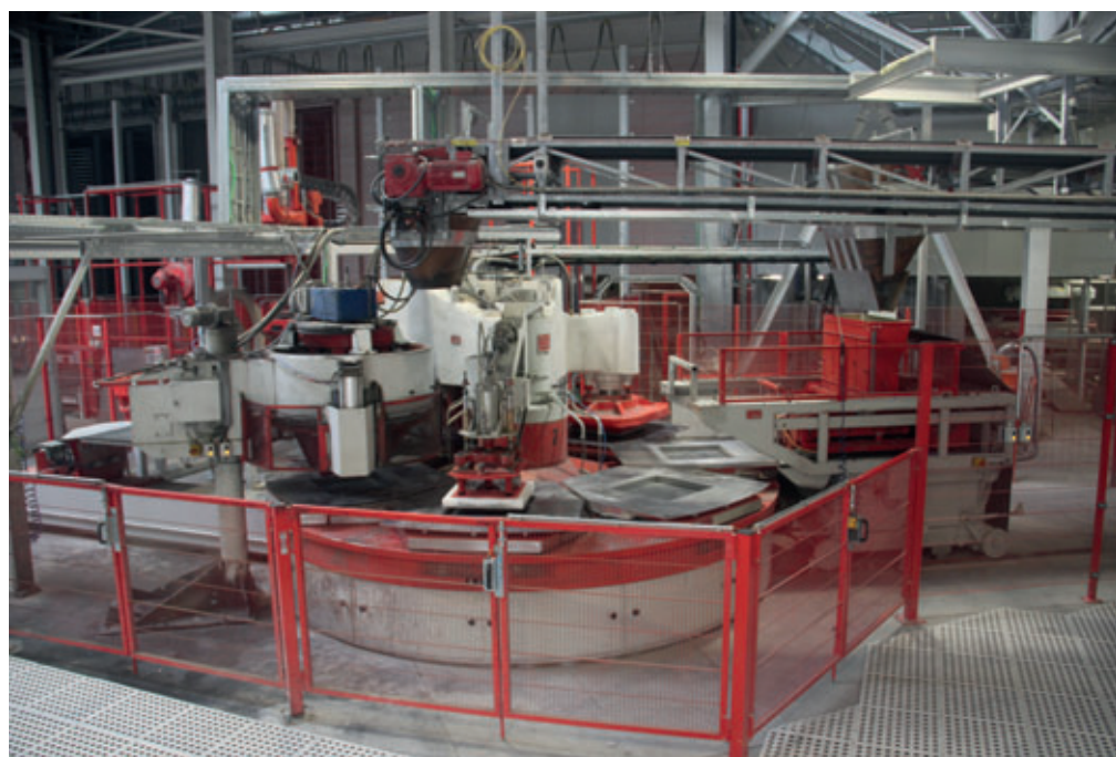
The hermetic press can manufacture formats up to max. 800 x 1,000 mm
