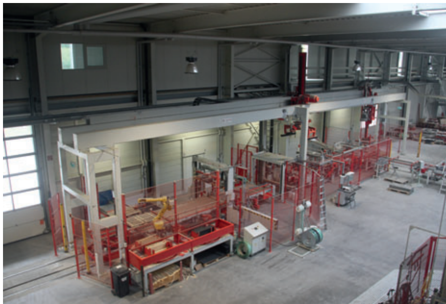
Flat/upright packaging unit with robot for the placement of wooden strips
