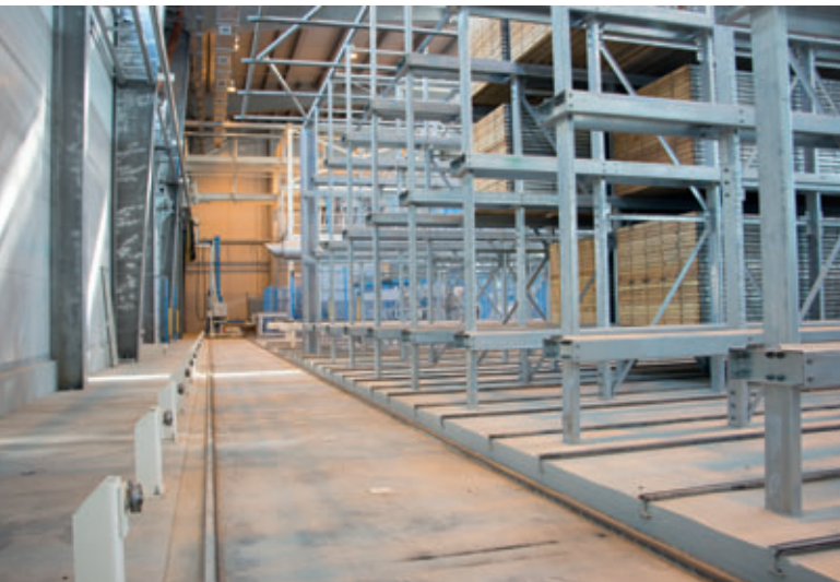
Depending on requirements the boards are either buffered or supplied to the production cycle
