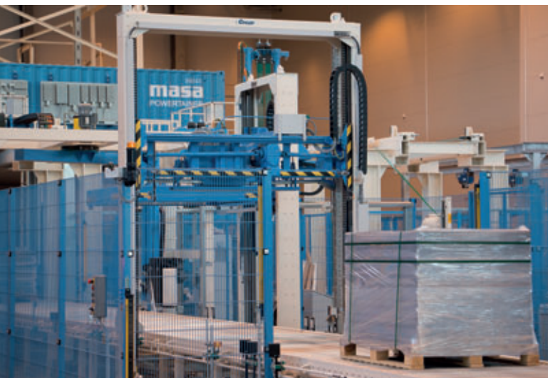
Well packed and ready for transport: foil wrapping plus vertical and horizontal strapping of the finished paving stones
