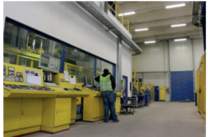
The XL 9.1 concrete block making machine can be observed through the window facade of the sound insulating enclosure
