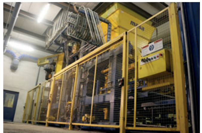
The new Masa XL 9.1 concrete block making machine at the Kann company's Leipzig plant
