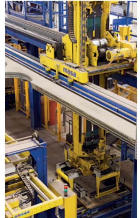
The Masa Cuboter has no hydraulic components; it uses exclusively servo drives
