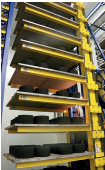
The distance between the forks is adapted to the product height
