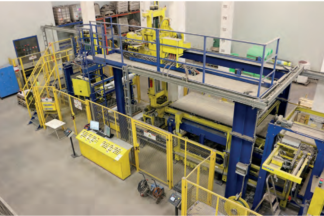
Dry side with remodelling for paving stones; production of garden and landscape construction products and kerbstones at optimum speeds
