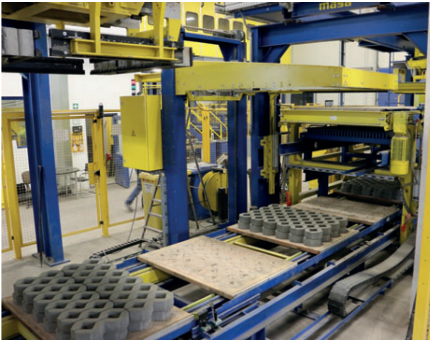
Horizontal strapping of individual layers – strapping takes place both on the return transport and during remodelling
