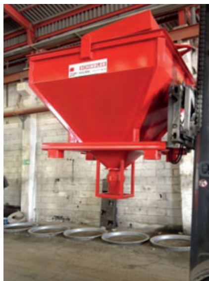
Thanks to the special dosing unit, segregation of the concrete on emptying is avoided as far as possible and the homogeneity of the concrete is retained.
