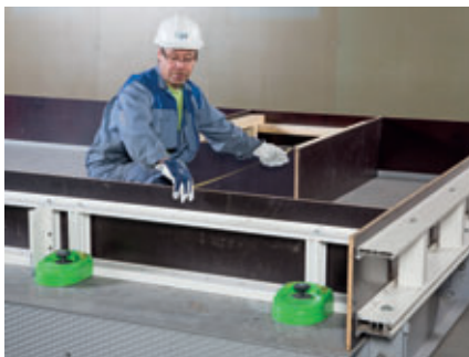
New addition to Elematic FaMe product family, the Flex-Pro side form for wall elements, sandwich panels and beams/columns up to 500 mm in side form height. With the Flex-Pro, the element is always straight with 90 degree corners. Flex-Pro is light in weight, 7 kg/m.
