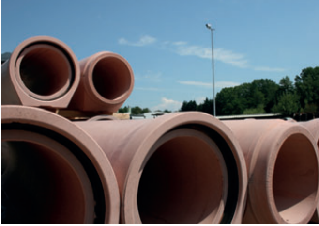
Even pipes in nominal width classes 2 and 3 are now manufactured as prebed pipes - DN800 concrete base pipes are shown in the image
