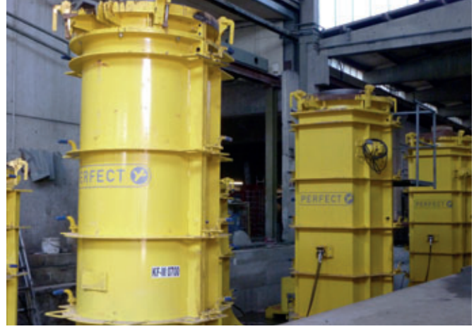
To produce pipes with nominal widths from DN700 to DN1200, Beton Müller commissioned multiple moulds in a lowered hall area
