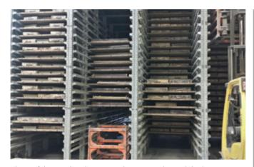
The prefabricated rack system solution was deemed the best approach because it incorporated the greatest amount of products in the smallest footprint, fit into one of the three the existing curing chambers, allowed for quick installation.
