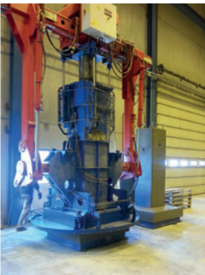
Demoulding at the curing station
