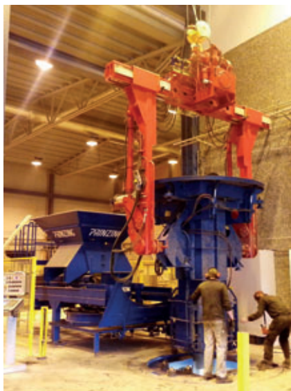
Atlas with turning spreader beam
